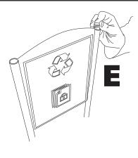
**1.6** Slide the assembled wallet down in between the tubes until the hooks on the edge of the wallet locate at the base of each tube slot (diagram D). 1.7 Place the two caps in position on top of each tube (diagram E).
