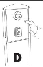
**1.5** The graphic holder comprises of a clear rigid wallet, a gray card infill and optional graphics. Place the chosen graphic in front of the gray infill. (a second graphic can be placed behind the gray infill so it can be visible from the rear of the unit).
