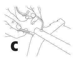
**1.4** Push the tubes upwards until they reach the base of the unit and the screws are held in the locating slots at the base of the unit. Tighten the fixing screw and nut using the wrench and allen key provided (diagram C).
